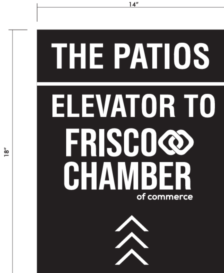
A DIRECTIONAL SIGN SCALE 1:2 QTY: 3 1/4" BLACK PAINTED ACRYLIC WITH 3M WHITE VINYL GRAPHICS. VHB TAPE & SILICONE MOUNT
